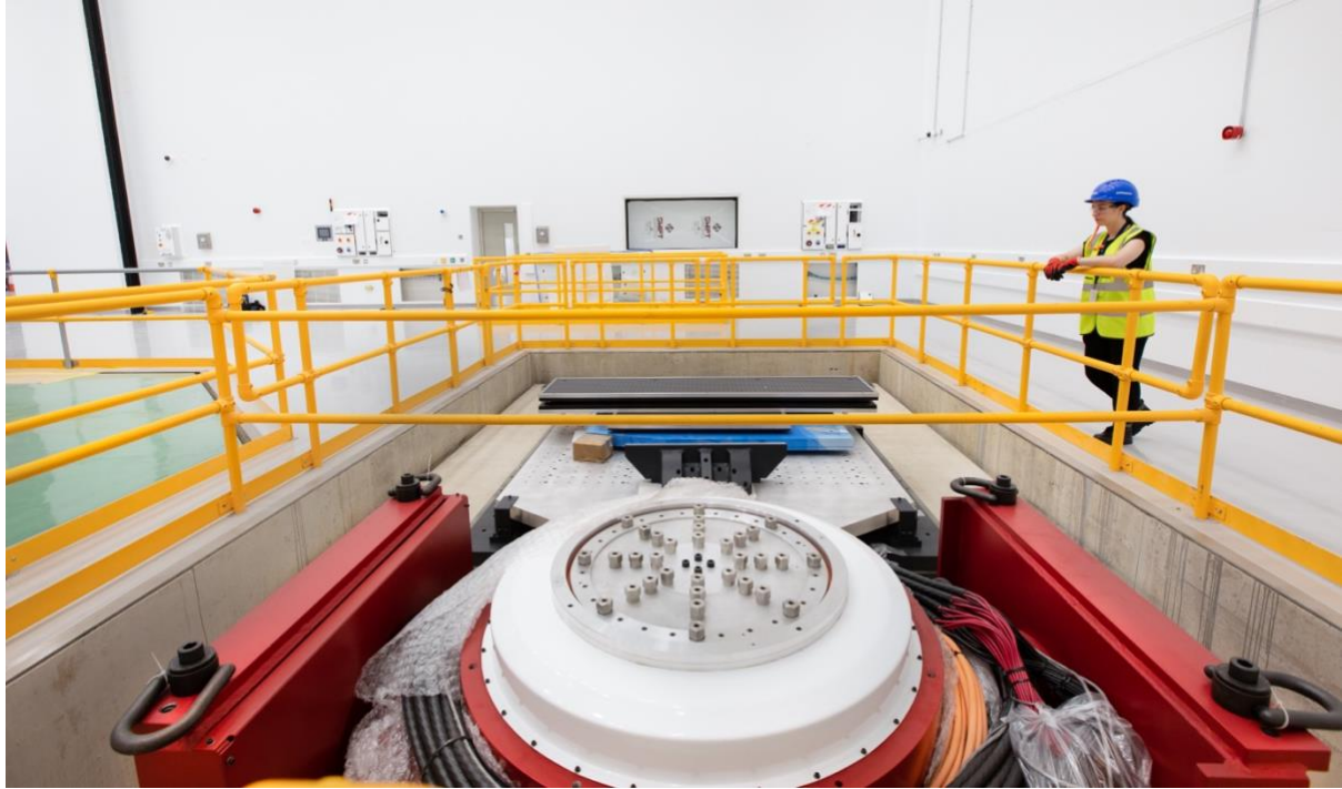
Figure 3 – The NSTF Vibration Suite undergoing construction. Credit: STFC RAL Space.
